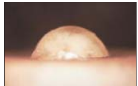
Fig 4 Wetting test: Unfavourable wetting (top) and wetting of the CBN-equivalent surface with the HPB bond (bottom)
